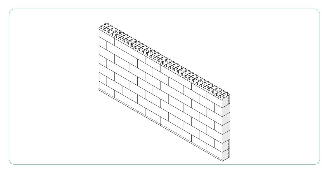
$\label{lockblock} \mbox{Completed straight section of QUICKBLOCK wall with fixing plates.}$
