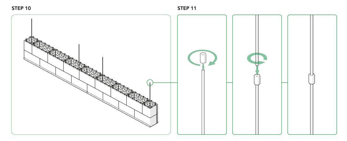
Once the first length of threaded rod has been attached to the fixing plates, construct the first two layers of blocks.
