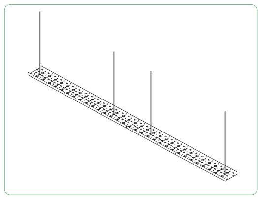
We recommend using a minimum of 2 connection points per length of fixing plate, this will give sufficient tension to the wall once completed.
