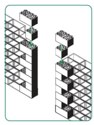
Now, replicate this bricklaying pattern until the structure is nine layers high, remembering to use **Half Blocks** every second layer.
