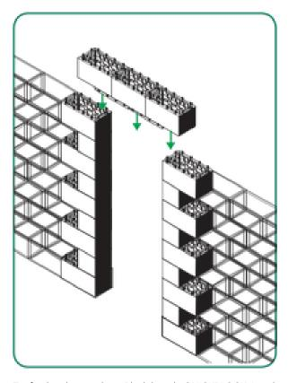
To finish, place a three-Block-length QUICKBLOCK Lintel structure\* on top of the opening. The lintel should be placed such that it completes the bricklaying pattern, and the QUICKBLOCK **Capping Pieces** sit flush with the sides of the opening.
