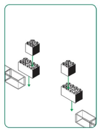
The configuration of the bottom layer determines the location of the door space. Where desired, remove two **Full Blocks** from this layer.
