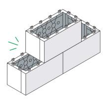
Opening blocks with excess force may result in blocks becoming damaged. It is recommended that blocks are opened with two hands and moderate force. QUICKBLOCK does not accept responsibility for blocks that are broken due to user error.
